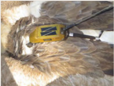
Close-up view of a GPS tag on the back of a live vulture.
