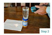
3. Turn on the flashlight and shine the light through the clear glass full of water onto the white piece of paper. This is the tricky part. This part of the experiment is called trial and error. You will need to adjust the angle of the flashlight and how close the flashlight is to the glass until you see a little rainbow.
